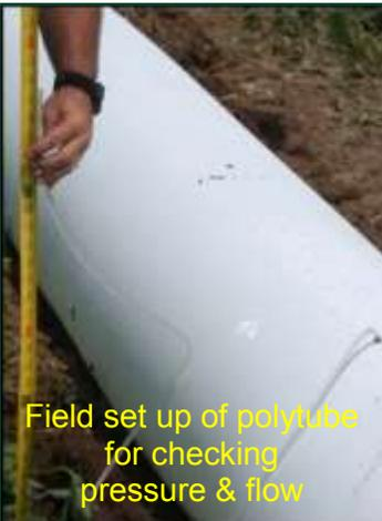
Field set up of polytube for checking pressure & flow
