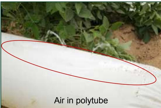
*Occurs when the wrong size (diameter) and thickness (mil) of polytube is used. Air pockets in the polytube can also add to this issue and cause bursting.*
